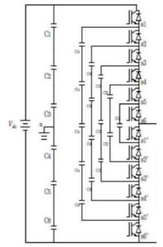
Fig. 3. Seven level capacitor clamped inverter
