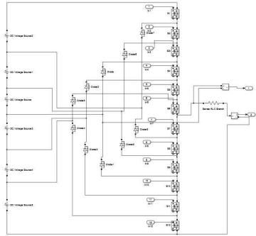
Fig 8. Simulink model of NPC MLI
