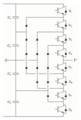
Fig. 2. Seven level diode clamped inverter[5]
