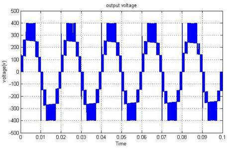
Fig. 9. Output voltage of new topology with seven levels
