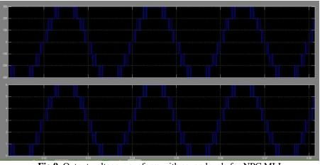
Fig 9. Output voltage waveform with seven levels for NPC MLI
