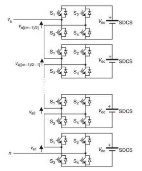
Fig. 1. Structure of a multilevel cascaded H-bridge inverter[2]
