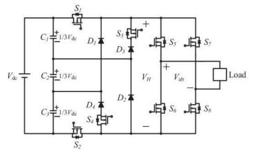
Fig. 4. Seven level Inverter with reduced number of switches[3]
